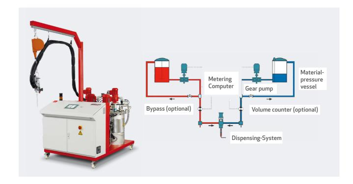
The eldomix 600 is a solvent free gear metering and mixing system, used to handle low to medium viscosity multi component media, such as epoxy resins, polyurethanes or
